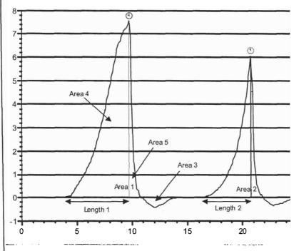
A typical force-by-time plot produced by an Instron 888 with a Warner-Brazler head used to determine texture profile characteristics objectively.
